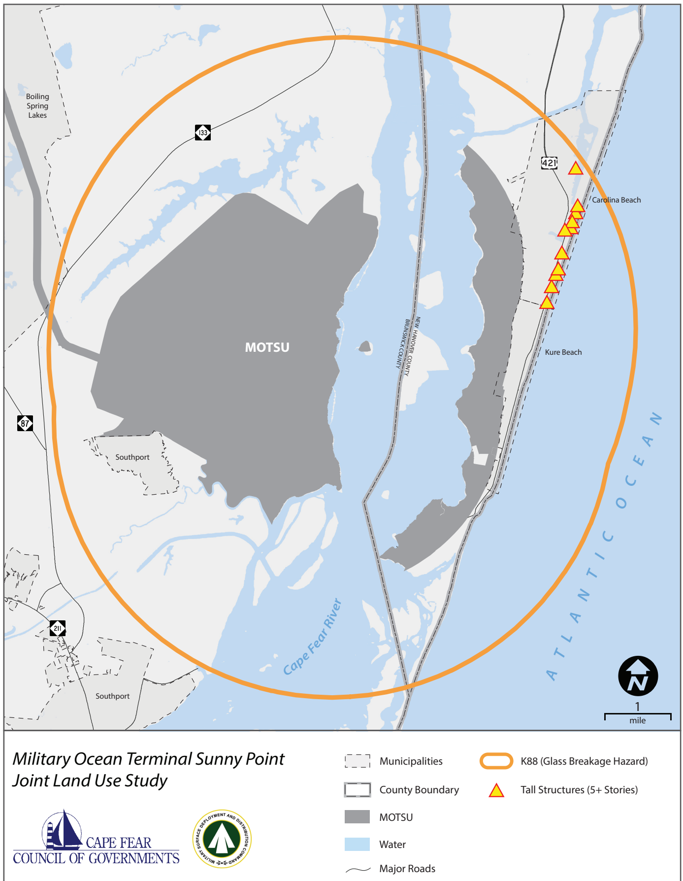
Figure 5.4: K88 Glass Breakage Hazard ESQD
